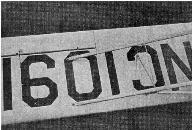
Wing strut attachment to wing – note servo access hatch.
