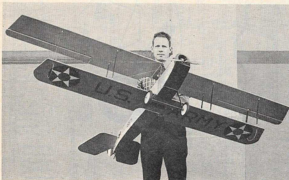
Author explains that wing tip skids are as important on model as on real Jenny. On grass, all ground handling is easy with the effective, steerable tail skid. However, it takes practice on hard surfaces. Tip skids prevent wearing out wing tips!
