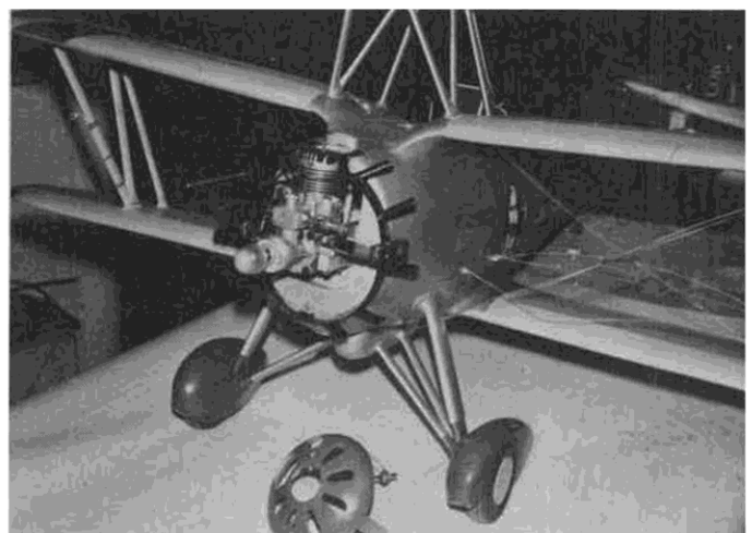
There's the Enya! Note exhaust ring. Fuselage is strip-planked over bulkheads. Shroud (foreground) is made from balsa.
