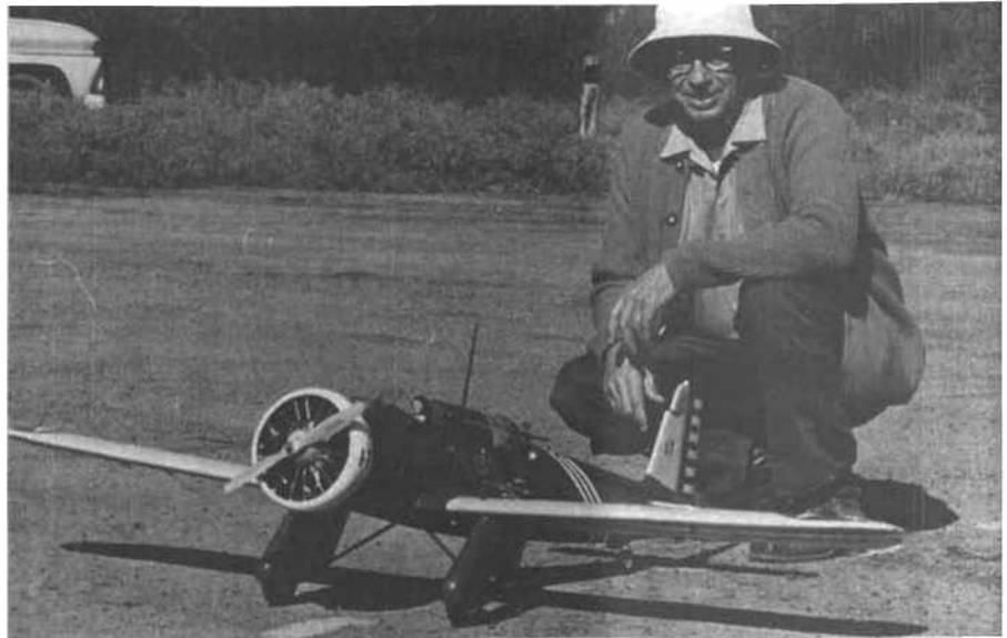
Charlie Smith and his dual purpose 'Shrike.' Note lead-out wires . and guide plate near lei: wing tip. Flying prop just about clears ring cowl. Radio gear remains aboard for U/C flights.
