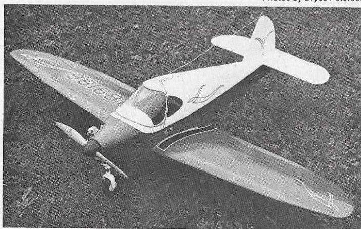
A side mounted Enya .29. Fuselage is narrowed slightly, close to scale. At left: "Culver" in the foreground, a Mooney M-18 keeping it company. Below: Dihedral tips were a unique touch. An M-6 foil, hardwood spar.
