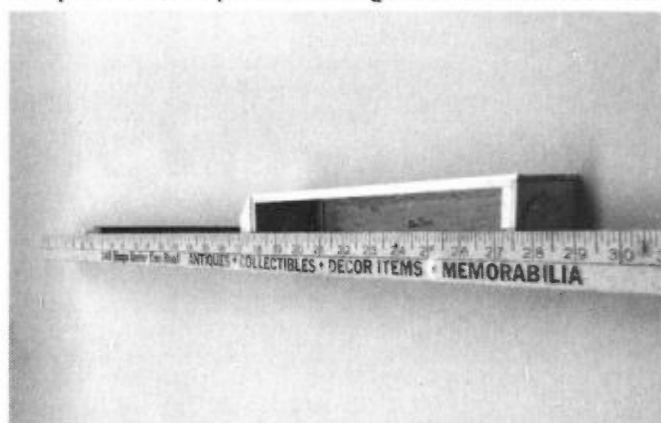
LEFT: Use straightedge to align boom with fuselage. RIGHT: Make up stabilizer mount using 1/8" balsa base and 3/8" balsa triangular stock. Align the stab mount so that it is square with the wing mount, and glue in place using CA cement.
