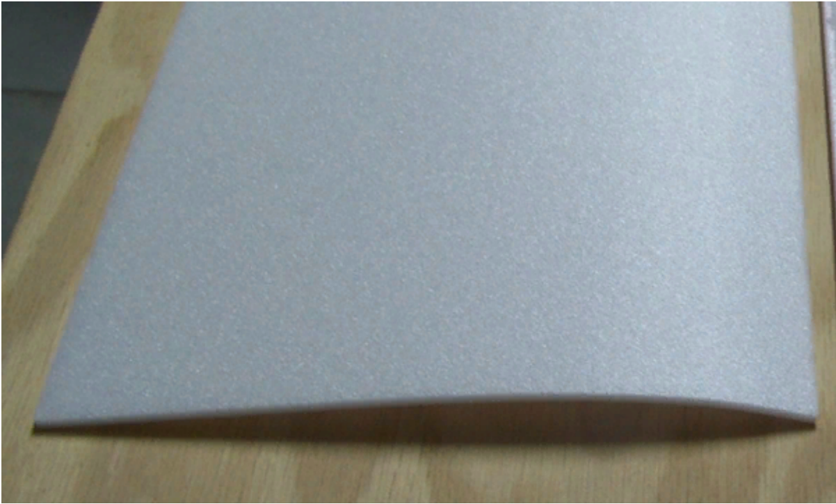
Roll form the top wing skins using a broom handle or 3/4-inch dowel.
