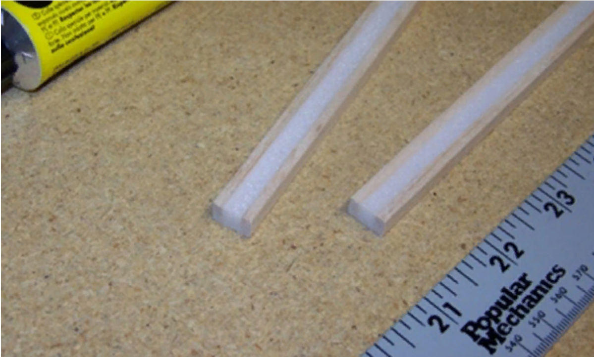
Wing spars are made with 6 mm foam sandwiched between two balsa sticks.
