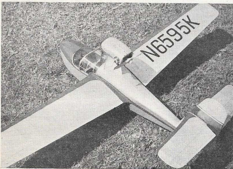
The spacious cockpit of the Skimmer provides scope for plenty of interior detail and cancels out the need for ballast.
