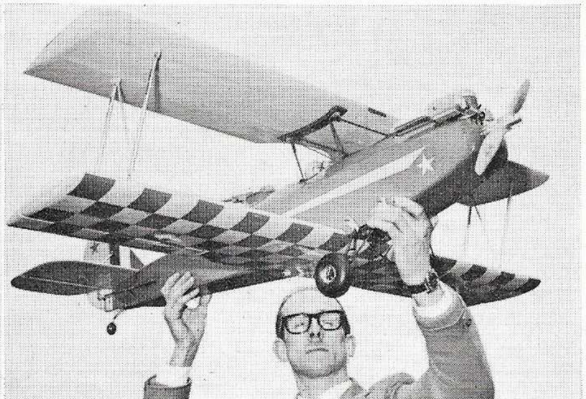
Below: two views of the underside, emphasising constant chord wings. Ailerons on bottom wing only. Note checker-board finish—good example of what can be done with those iron-on covering materials.
