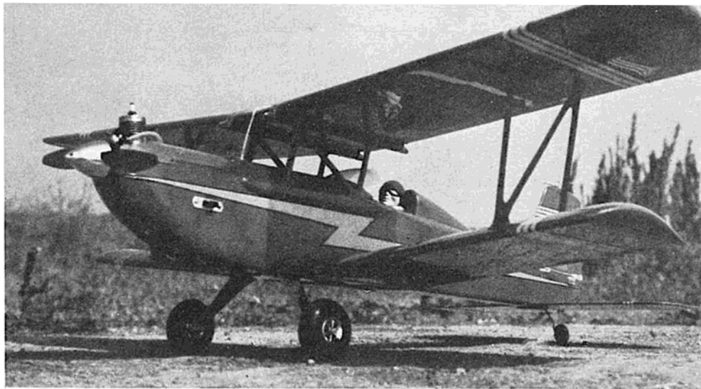
All sheet construction, O.S. Max .10 or .15, super MonoKote finish, a small digital system, and some weekend flying fun characterize Ken's Classmate.
