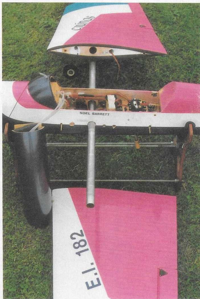
Left: Equipment bay, showing servo layout and tank installation in the canopy. Below: Sturdy 7/8" wing tube soaks up the flying stresses. Wings feature variable incidence for fine trimming.
