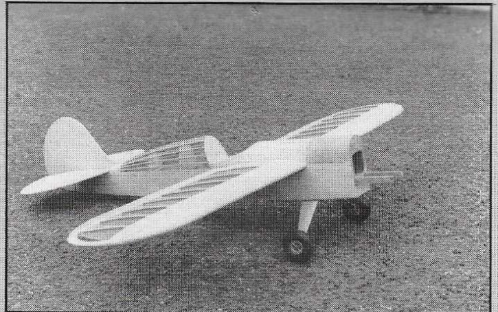
All that is missing from this photo of the uncovered complete airframe is the built up cowling.
