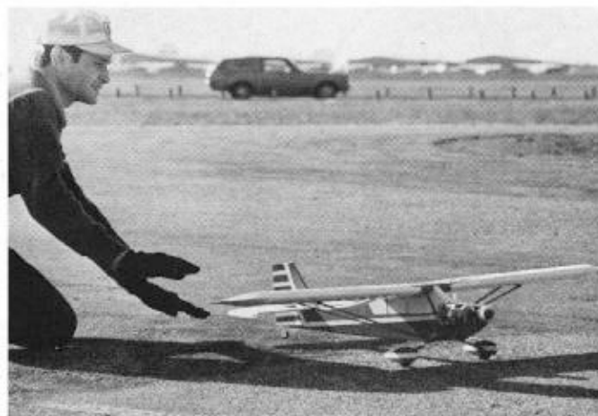
At left: Matt Smith does honors as Rick applies a shade of "up-elevator" to unstick it. It's lightly loaded for the power, so it almost jumps up. Below: Past practice has been to bring leadouts from center of the mass.
