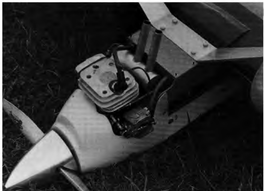
Gene's model used the Sachs-Dolmer 3.8 powerhouse, and even at an all-up weight of 23 pounds, his model flew great. Part of the weight came from the smoke system which Gene installed.
