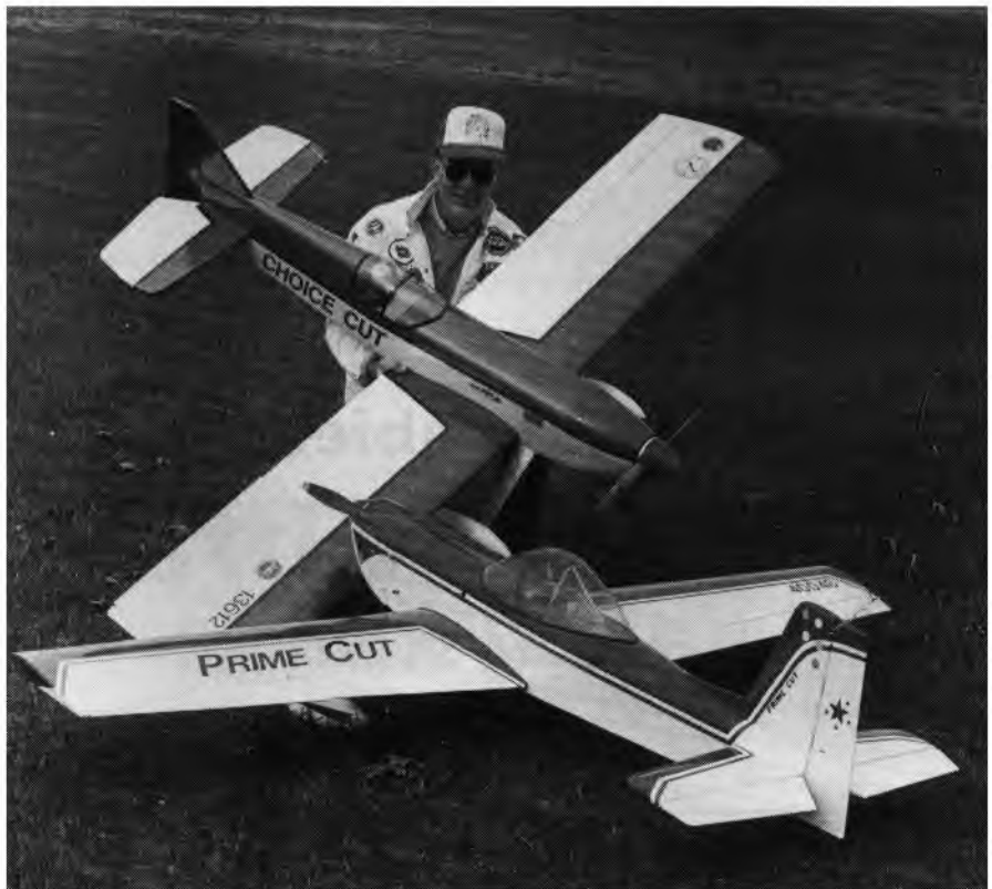
Compared to the Prime Cut , the Choice Cut , which Dick holds has a narrower, sleeker fuselage. The span is 90 inches with a 16% thick, symmetrical airfoil. Wing area calculates to 1440 square inches.
