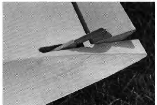
The bracket is cut from sheet aluminum, then bent. The lead weights bolt on. When the aileron goes down, the weight nests in a cut-out pocket ( above right ).
