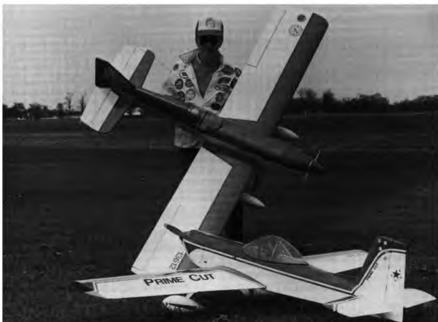
The Prime Cut , on the ground, was the sire of the Choice Cut which Dick holds. The primary differences are the no-taper constant chord wing and the narrow turtle deck of the Choice Cut .
