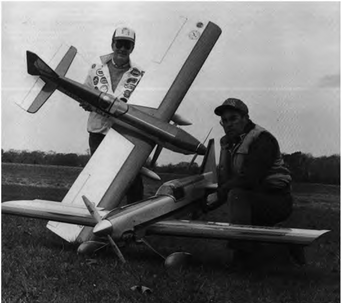
As Dick (standing) and Gene (kneeling) pose with their planes, the thick constant chord wing and conventional ailerons are very evident.
