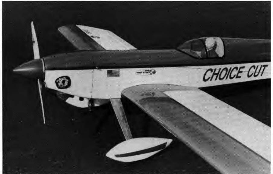
Some parts of the Choice Cut have been borrowed from Dick's P-51 Mustang . The streamlined cowl comes from it, as does the optional squared-off canopy. A 4-inch spinner fits nicely.
