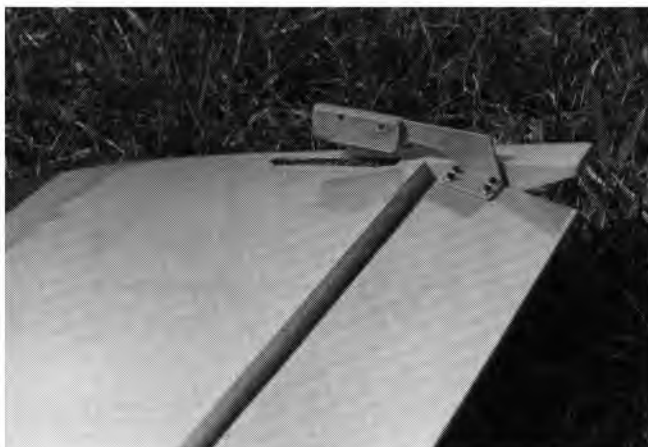
With larger engines like the Sachs, flutter could be a problem so an aileron counterbalance ( above left ) on the bottom of the aileron should be considered.
