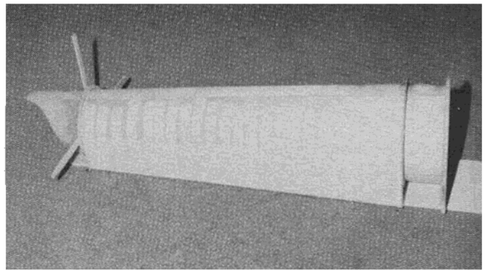
Sides held in place on tail pipe with masking tape while epoxy cures.
