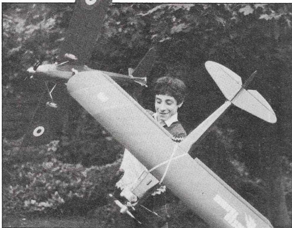
A brace of "Chickens"; two of the prototypes (photographed in 1983). Larger ailerons (1⅙ in.) on Ian Badls' example proved better than narrower ones on Dad's.
