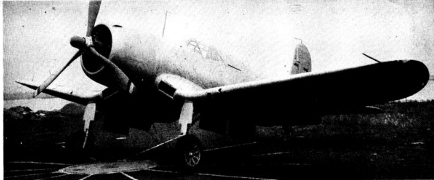
Prototype XF4U-1; note forward location cockpit (compare to plans below) and cowl guns.
