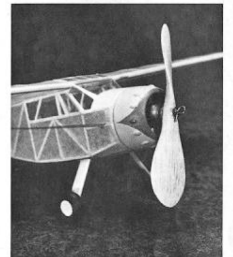
Hold your weight down aft. A laminated outline, strip stock for ribs. It tends to resist warps. At right: A hand carved balsa prop will improve performance. Cut it from a block per the blank. Below: It will just sit there until you pack it full of winds. Prop will screw it into the sky.
