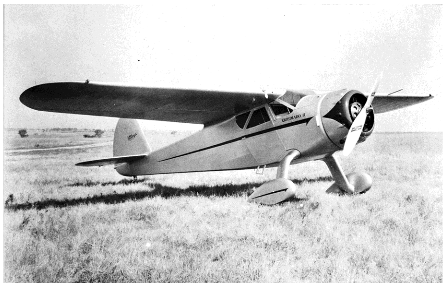
This C-145 was aluminum with Deep Vermillion trim and Marine Blue pinstripe. Third C-145 built (note perforated plate between prop and cylinders) was sold to Ignacio Ogueira of Rio de Janeiro and then registered PP-TEH.
