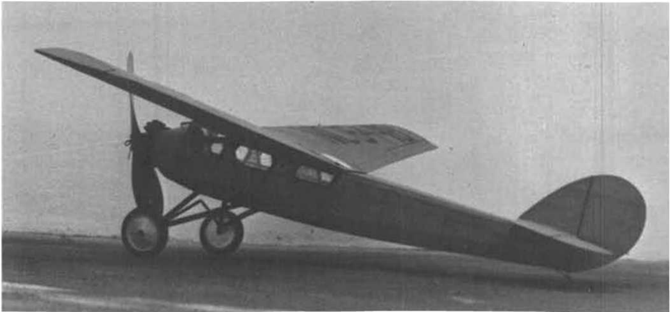
Long tall moment adds to ground and air stability of the Cessna. Original was one of earliest light passenger types to use cantilever wing structure ... no struts.
