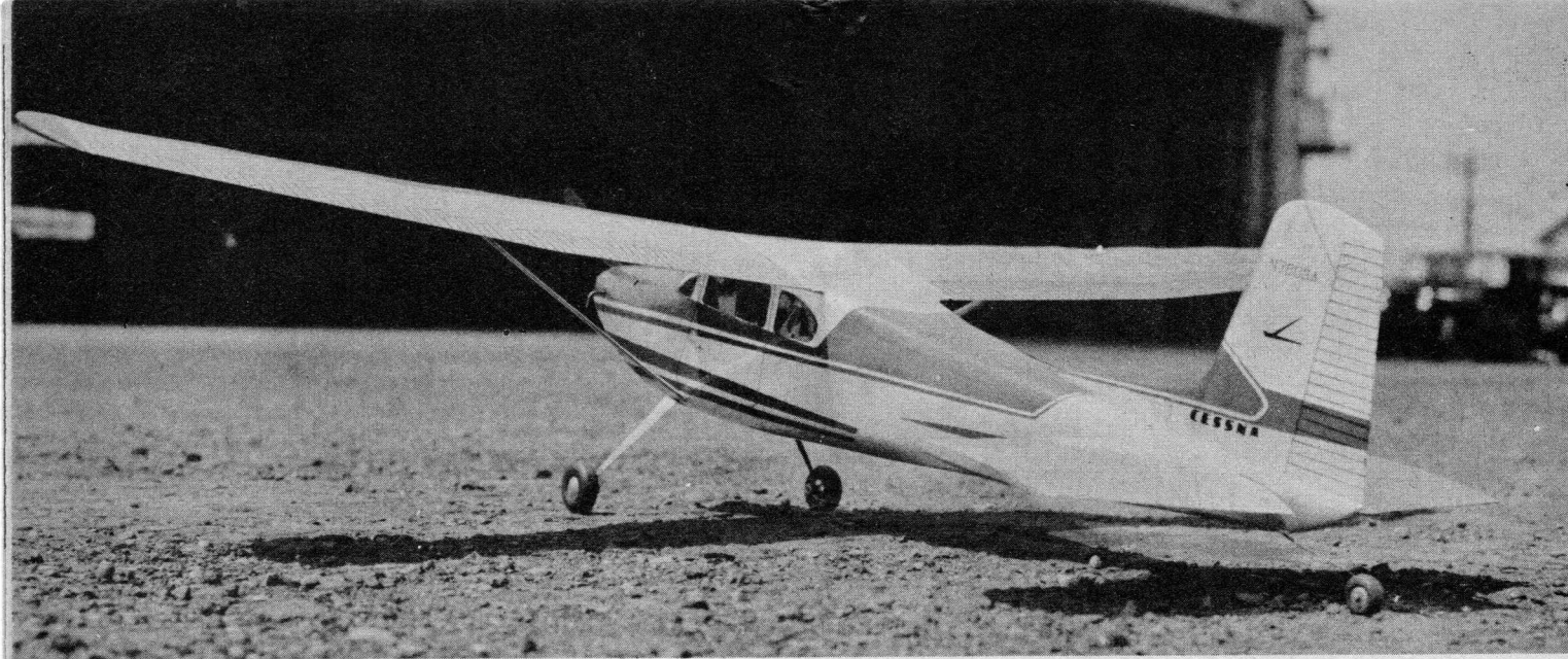
Two-piece wings detach, just like the real thing. Requisite for metal covering is liberal use of Sanding Sealer and a velvet smooth sanding of wood.
