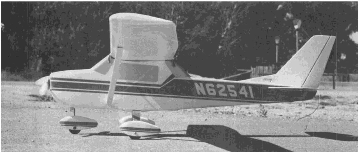
The simple-to-build square fuselage doesn't really detract from the overall appearance of the model. Fred covered his in white Solarfilm and trimmed it with Monokote. Flying mags will give you all sorts of trim color combinations . . . or do your own thing.
