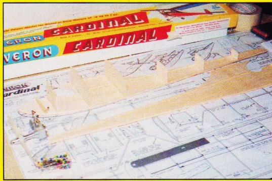
The fuselage side is trimmed to fit the plan and then the formers are glued in position making sure they are square.
