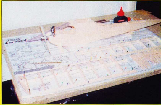
The wings and tail are built over the plan in traditional fashion. Make sure they are pinned down firmly to ensure a warp-free structure.
