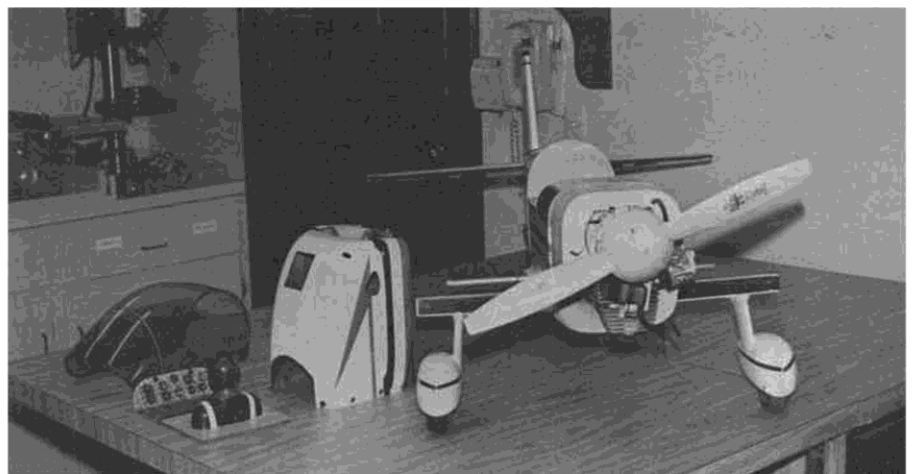
The combination wing beam and landing gear mount takes all flight and landing loads. It's eight laminations of 1/8 spruce laid up with epoxy. Canopy is molded plexiglass.
