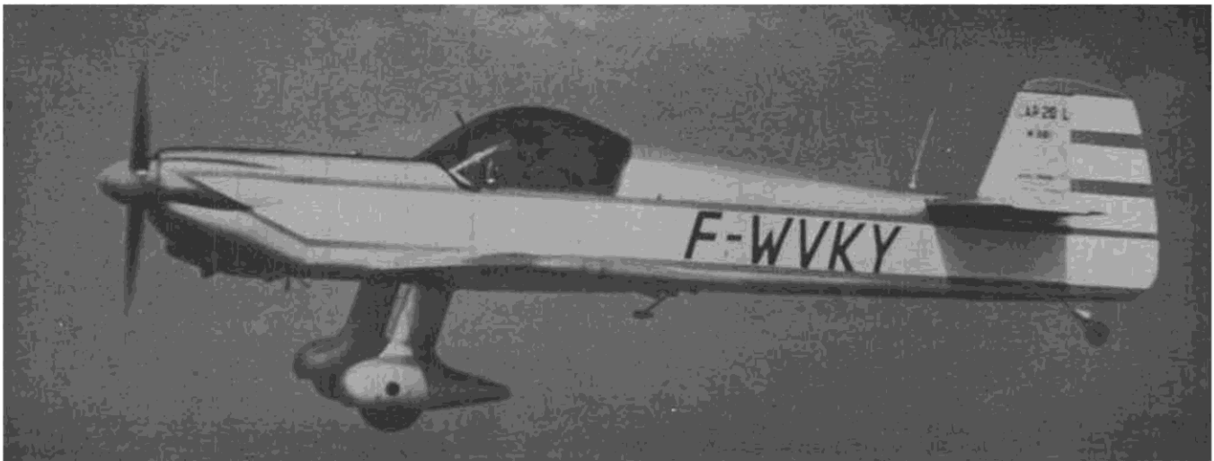
Flight shot of the full-scale CAP 20L, reproduced from company brochure. Ship derives its shapely fuselage and distinctive wing planform from the French Emeraude lightplane. Jeff's model represents a 200-hp Lycoming powered version.
