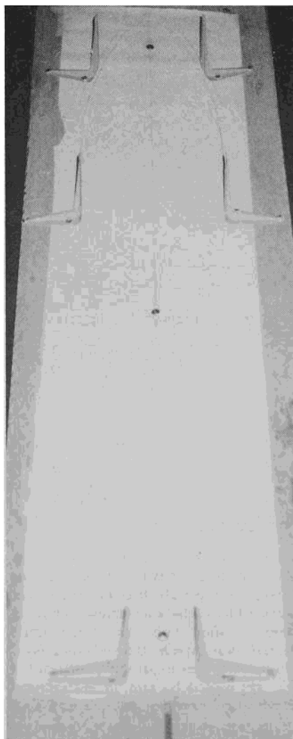
Simple jig using 4" shelf brackets ensures that fuselage is built straight.
