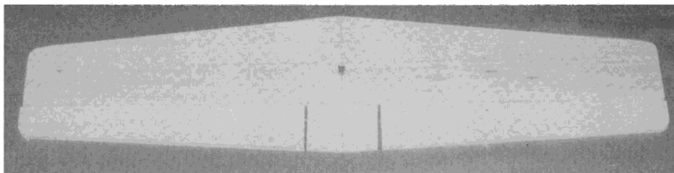
The horizontal stabilizer and elevator are cut from 1/4" balsa sheet.
