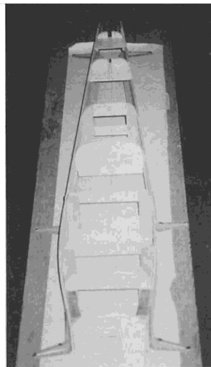
Fuselage in jig.
