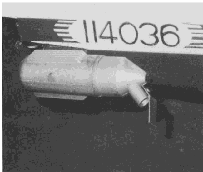
LEFT: Simple air deflector made from 1/16" aluminum prevents excessive back pressure at exhaust outlet. RIGHT: Bottom view of completed aircraft.
