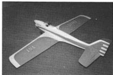
Note the symmetry of shapes for the wing, stabilizer, and rudder planforms. Lines blend together nicely.
