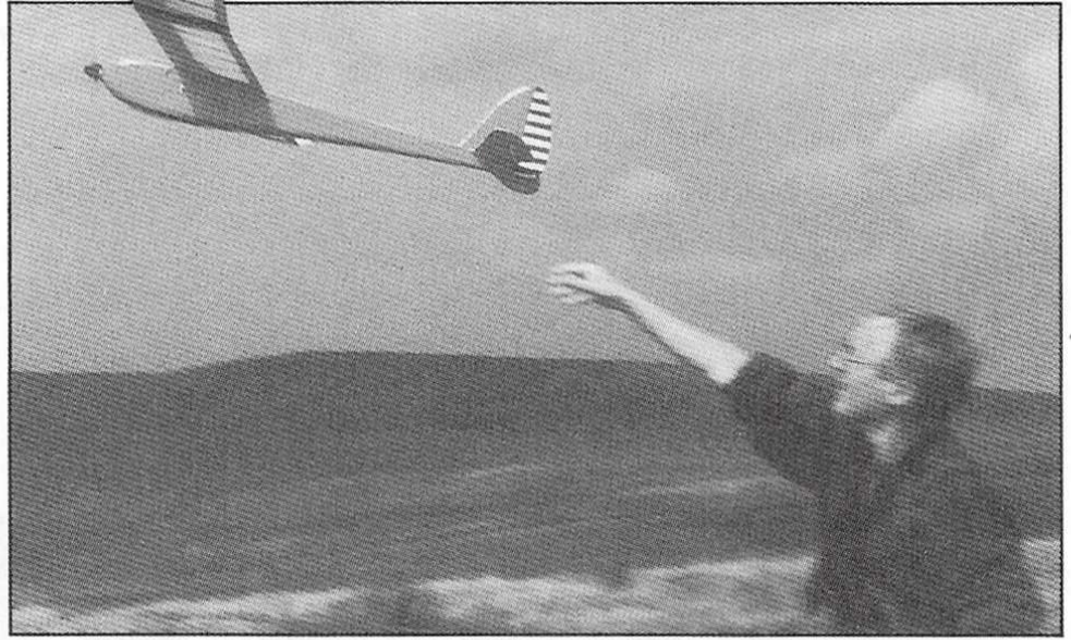
Away she goes! Average flight times are in the 20 minutes range on six cell 7.2v power.
