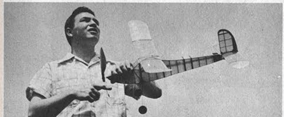
Hand winding for a short test flight, the author uses a contest-type folding one-blade prop.
