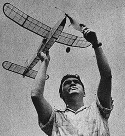
How to hand launch: release prop, then gently push ship forward. Don't push up into stall.
