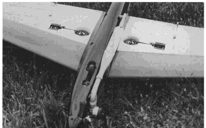
Underside shot shows Southern R/C retracts, pipe mount, and aileron pushrods. Monokote on wing and stab saves mucho weight.
