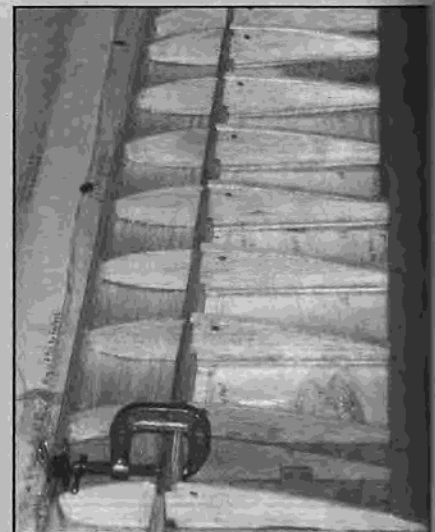
Gluing LE and spar joiners to first wing panel.
