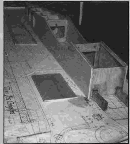
Bottom crutch and hatch cover before installation.
