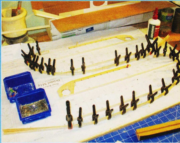
TOP LEFT: An added bonus of this style of construction is that servos can be fitted while there is still easy access. TOP RIGHT: Fuselage sections joined and the selection of batteries Pat had to choose from. Along with the remaining hardware. ABOVE LEFT: Lots of clamps used to assist with laminating the wing leading edges. ABOVE RIGHT: Scale rib/sub-rib count makes for a 'busy' looking wing. Ply plates are for aileron servo attachment.
