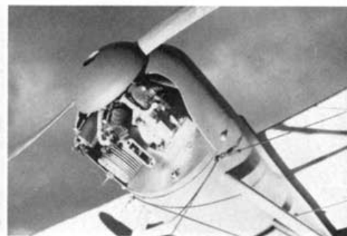
Buried behind the cold and phony dummy engine, one that provides the life. The cowl design is a natural for such realism. Engine cools well.
