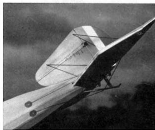
Fin and rudder from \frac{1}{4} " sheet, edges rounded. Photos will help you with placement of rigging. Below: Stab, elevators and streamlining seen.
