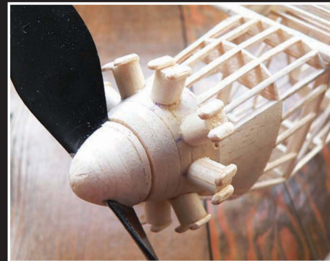
My dummy engine was very simple, and made up from scrap balsa. Pushrods would help with scale realism, it depends how far you want to go.
