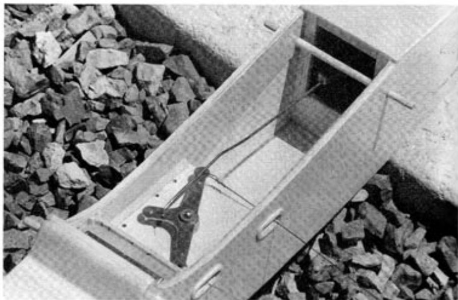
One nice feature of a two-piece stunt ship is easy access to the bellcrank. Note both the ample holes for the leadouts and the plywood doubler which tapers all the way back to the wing's trailing edge.
