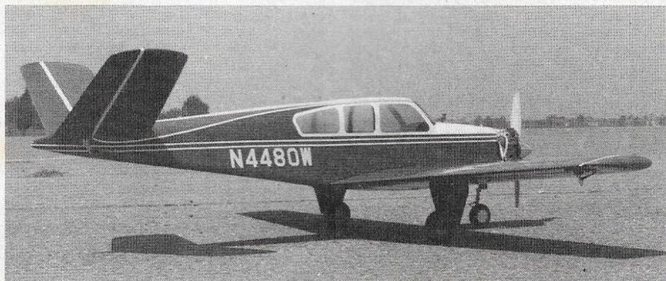
Author's Bonanza on the runway. Paint scheme is from actual plane owned by H.A. Sessions of Lubbock, Texas. Finish is K&B epoxy paint and surfacing resin. Distinctive "V" tail evident here. Pretty plane.
