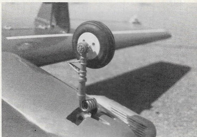
Wing mounted landing gear leg (above). No retracts, just fixed gear and wing mounted door. Nose wheel (below). Simple and effective. Aileron horn and pushrod (bottom). Uncomplicated hookup.
