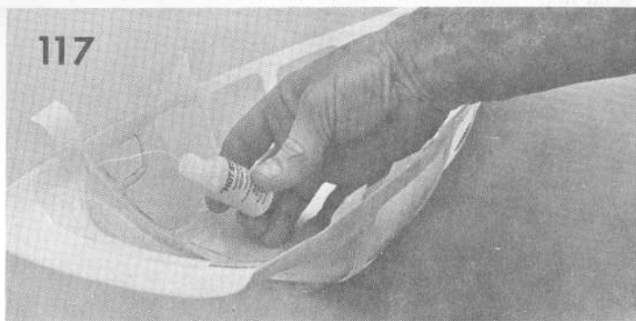
117. Position windows and put masking tape on the outside to hold the window in position. Start spot gluing with Hot Stuff or similar cyanoacrylate glue, front and top of front windshield, work towards the back, be careful not to distort the shell, tack glue just a few places and try a check fit on fuselage before continuing.
