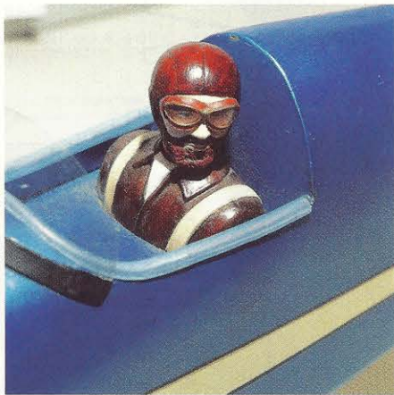
I personalized the Williams Brothers' 2-inch scale pilot with a little 5-minute Z-Poxy and 410 micro-light filler for the beard. Instead of gluing the head in place, I mounted it on a length of Sullivan Nyrod and attached it to the rudder servo. The cockpit combing is nothing more than silicon fuel tubing split lengthwise and pressed in place.
