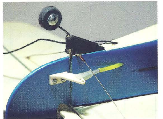
Left: I mounted two more servos in the wing center section to operate the flaps and ailerons. Note the offset attach points for the flap pushrods. This equalizes the motion between the two flaps. If separate aileron servos are used, you can lay the flap servo on its side to equalize the motion as well. Right: The Dubro tailwheel and bracket and wheel provide positive ground handling. I added the wire bracing after flying the model several times, purely for cosmetic reasons.
