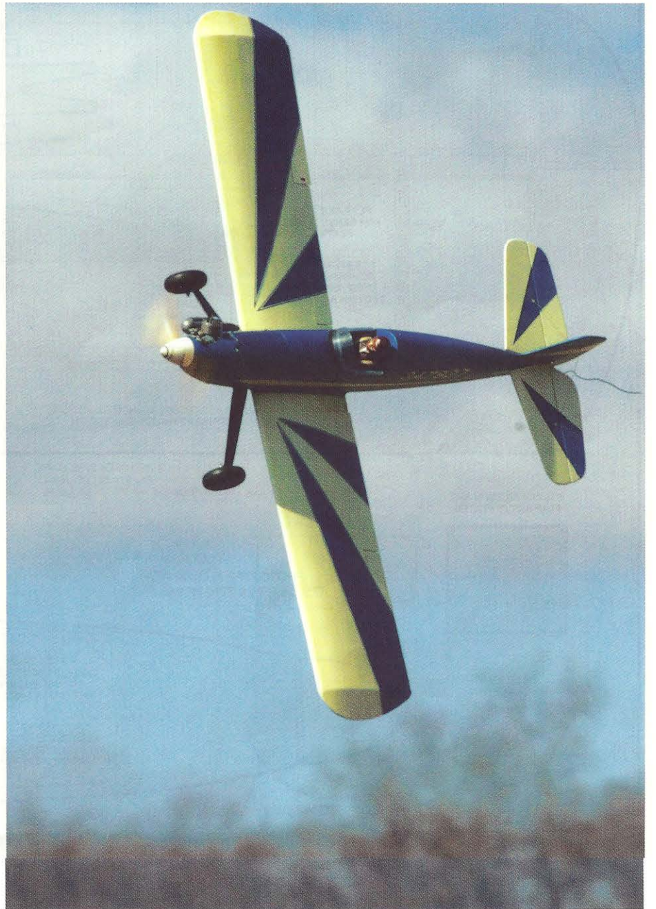
I personalized the Williams Brothers' 2-inch scale pilot with a little 5-minute Z-Poxy and 410 micro-light filler for the beard. Instead of gluing the head in place, I mounted it on a length of Sullivan Nyrod and attached it to the rudder servo. The cockpit combing is nothing more than silicon fuel tubing split lengthwise and pressed in place.
