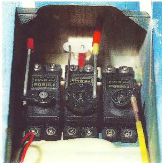
Three Futaba S-148 standard servos operate the throttle, elevator and rudder. Note the additional pushrod on the rudder servo to operate the swiveling pilot's head.
