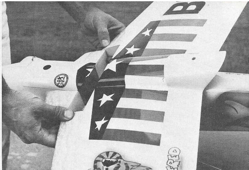
A wing slips into position. It's easier to mate the spar-like surface. A dowel holds all, bolt secure the rear. Structurally stressed for flight.
