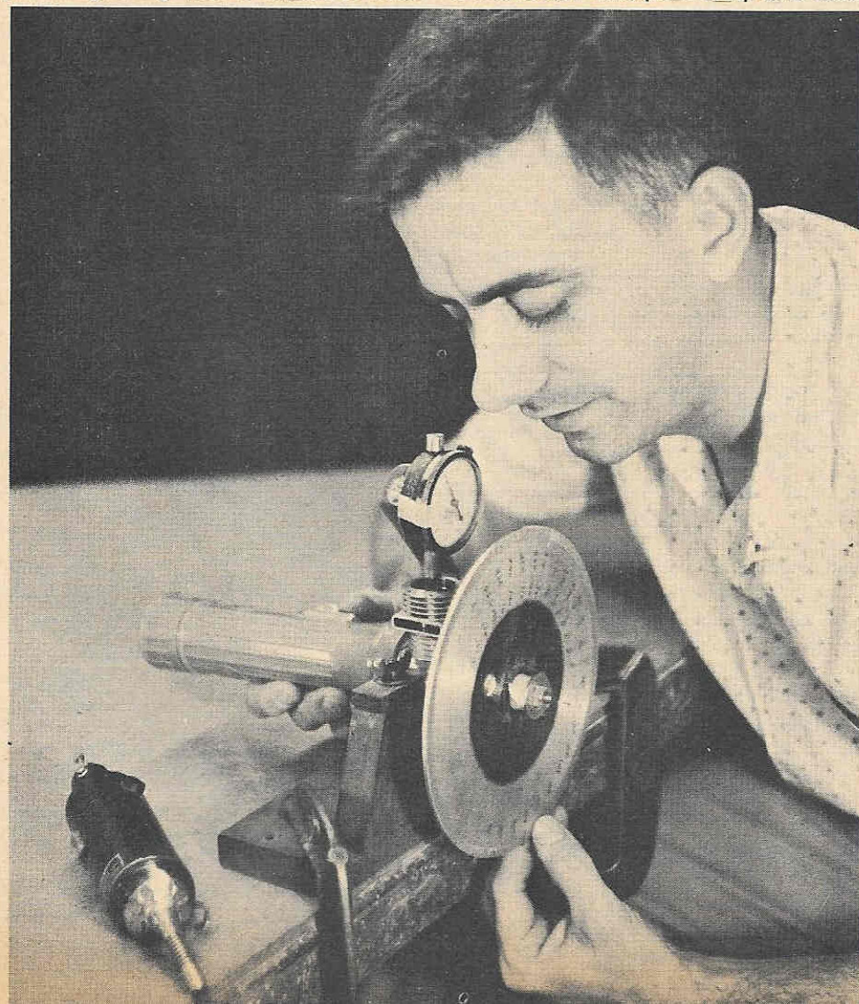
Using timing wheel and dial indicator to check port timing. Timing wheel is attached to crankshaft and indicates time cycle; dial indicator is used to show when piston at top dead center.
