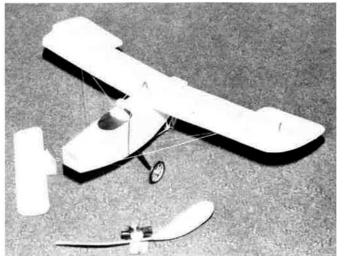
The little canard causes no problems in winding or replacing the rubber! Prop is made up of formed sheet blades on toothpick hub.
