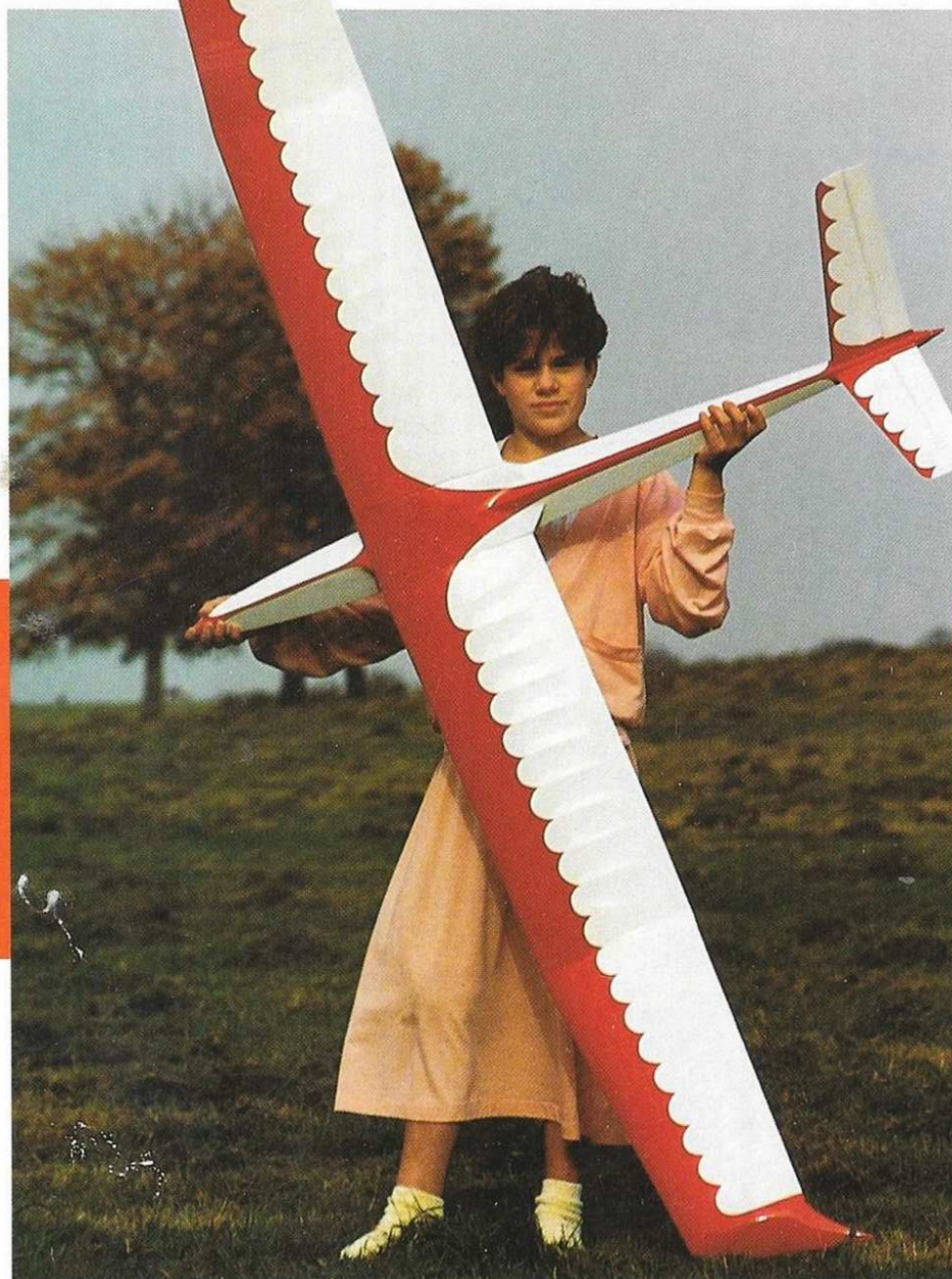
Vital statistics: span 96", weight 1775 grammes, wing area 5.75 square feet, wing loading approx 11 ounces per square foot. Looks good, too!
