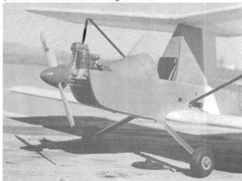
O.S. .20 4-stroke was installed with great results.
