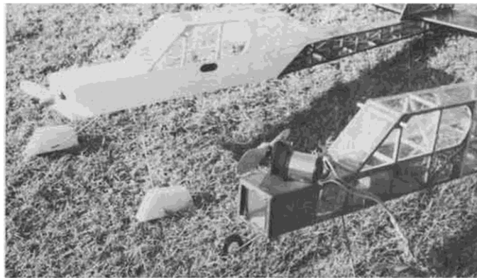
The Leisure Gear Motor is a perfect choice for the Big Bird . Removable ply motor mount plate makes motor installation a breeze.
