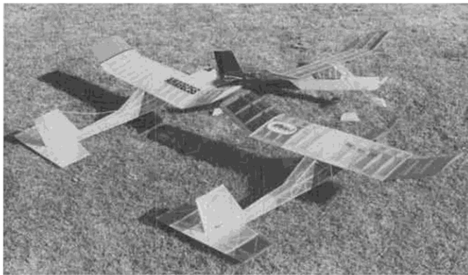
Big Bird the E.T. is a scaled up and modified Peck-Polymers Prairie Bird rubber powered model. Really shines as an electric trainer.
