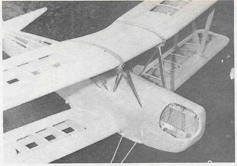
The upper wing is lashed on with rubber, not exotic, but really practical. Note the canted engine mount, it hangs the muffler way out in the breeze. Beneath: Engine turns a Top Flite 11-4 screw, gear is sold in hobby shops.
