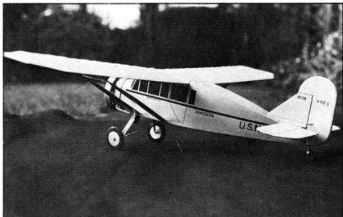
This little lightweight tips the scales at just under 8oz. ready to go! Film covering used on the prototype, insignia painted on white 'Fablon' and lettering and windows with Indian ink – matt polyurethane varnish fuel proofer.
