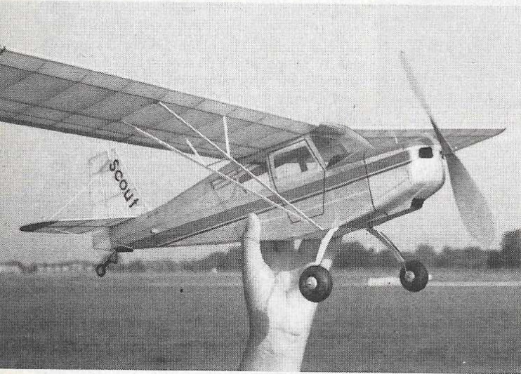
Scale details on the Scout help to pile up points in static judging (above). Door outline, stripes along side of fuse add to realism. Rudder and elevator are hinged with fine wire (below). Note tail wheel detail. Nice.
