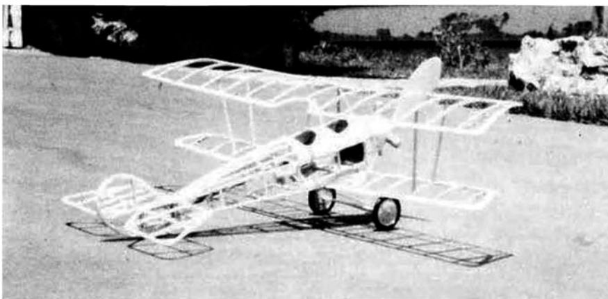
The Bellanca's bones show the simple, light construction. Wing leading edges are 1/16 dowel.
