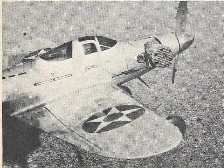
View of nose section shows angular arrangement for throttle linkage.
