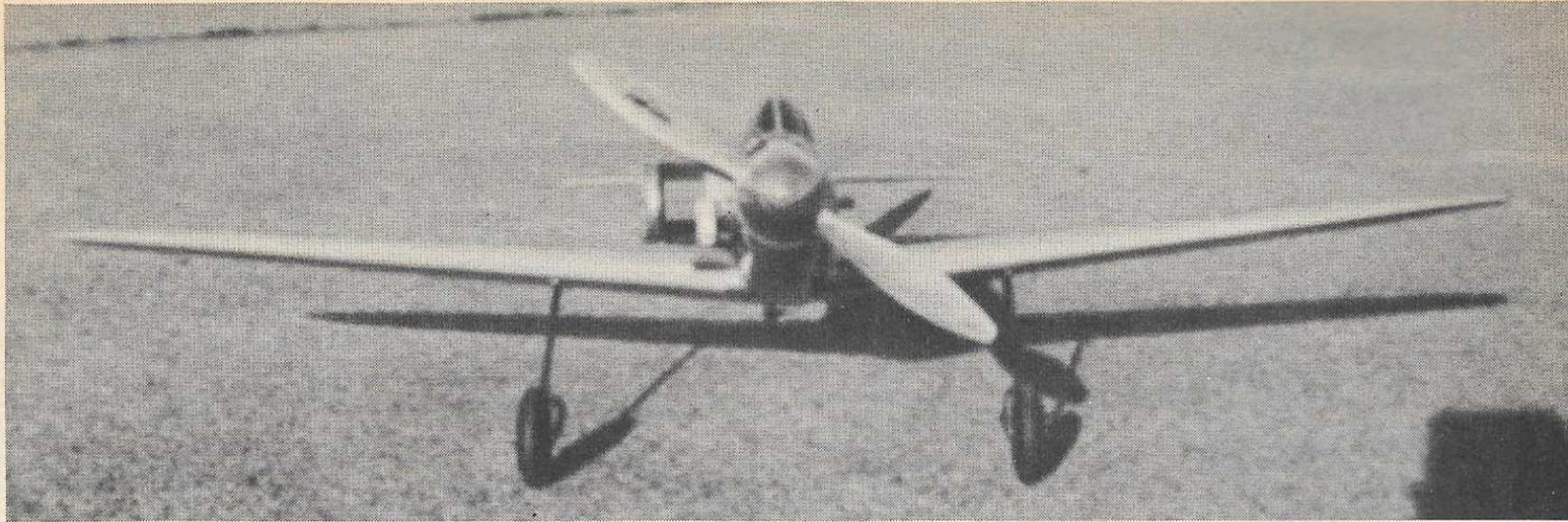
Head-on view shows compact, smooth lines. Actually, the engine dwarfs the nose of the plane. Short but springy landing gear helps hard-deck landings.
