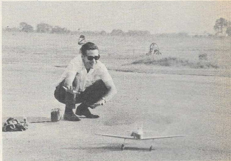
Good clean release for take-off. Note angular deflection of landing gear.
