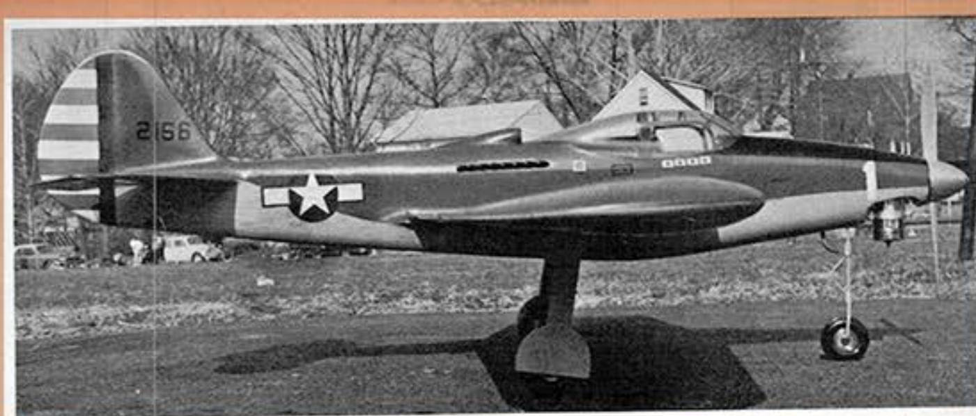
The Bell Aircobra design first appeared around 1939, was followed in WWII with the King Cobra, which lathered in armor plate, won fame as the "Flying Pinball". When struck with target fire, the nose lit up to score for attackers. First of fast fighter types.
