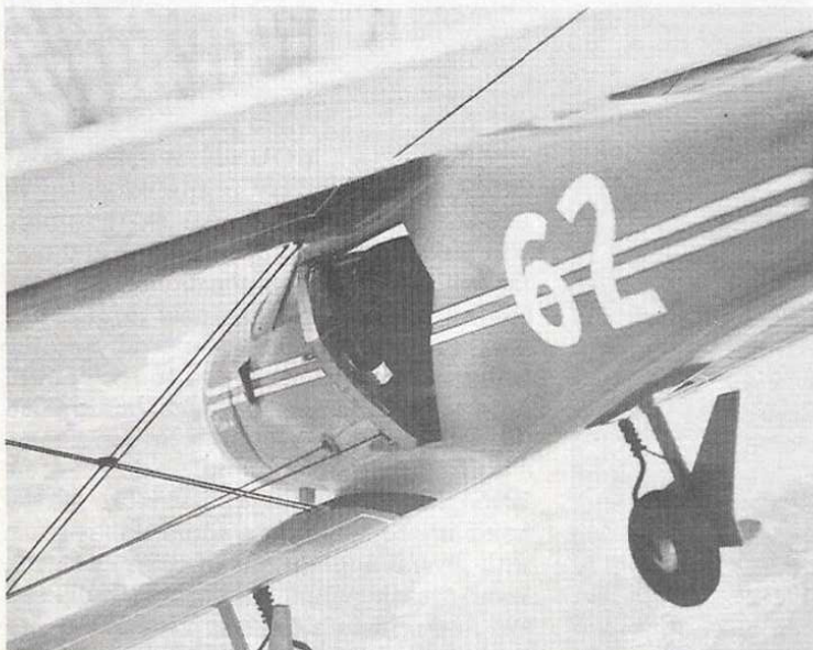
Note thin aluminum sheet latch to hold cabin door when it's closed.
